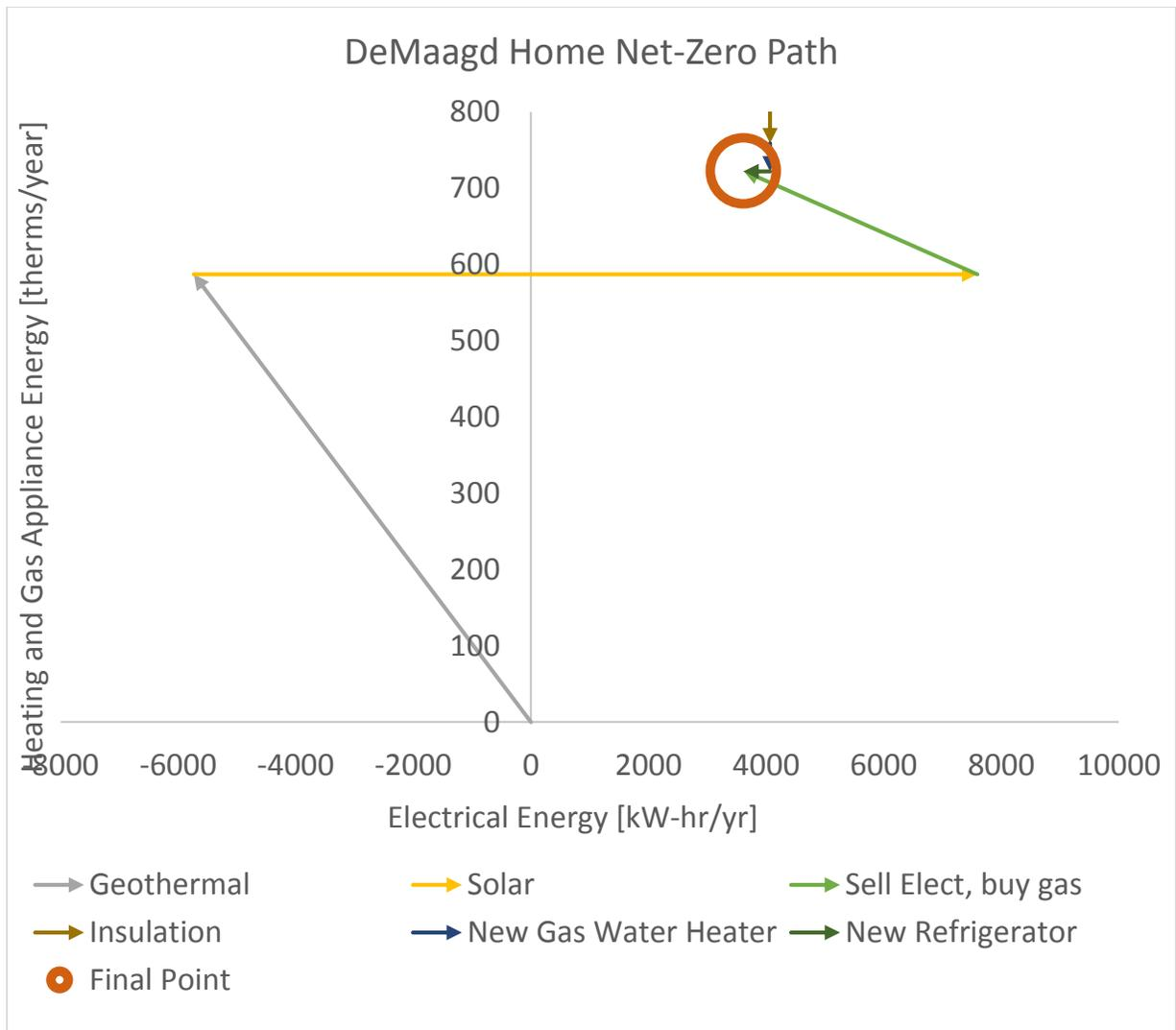
**Figure 15:** Combined energy saving/production path to net-zero home
