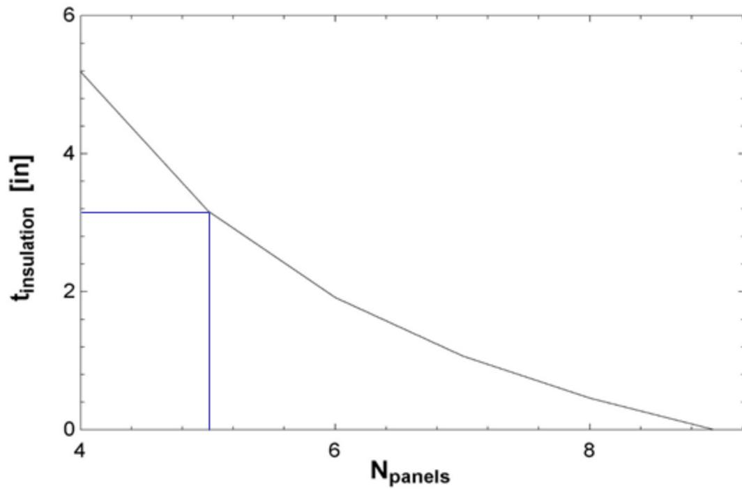
Figure C6-58. Combination of solar-heating panels and insulation needed to cover heating needs
