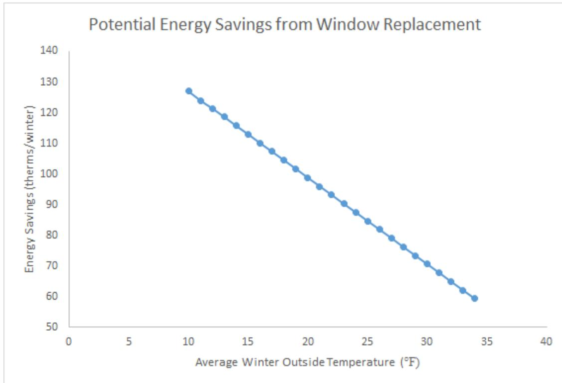
*Figure C6-57. Effects of outside temperature on savings from window upgrade*
