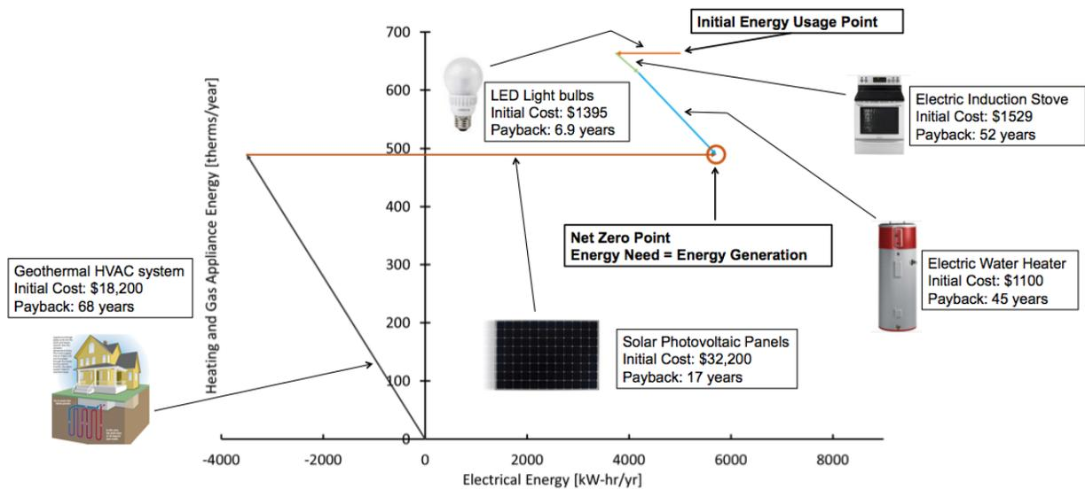
Figure 10: Overall Energy Reduction and Production
