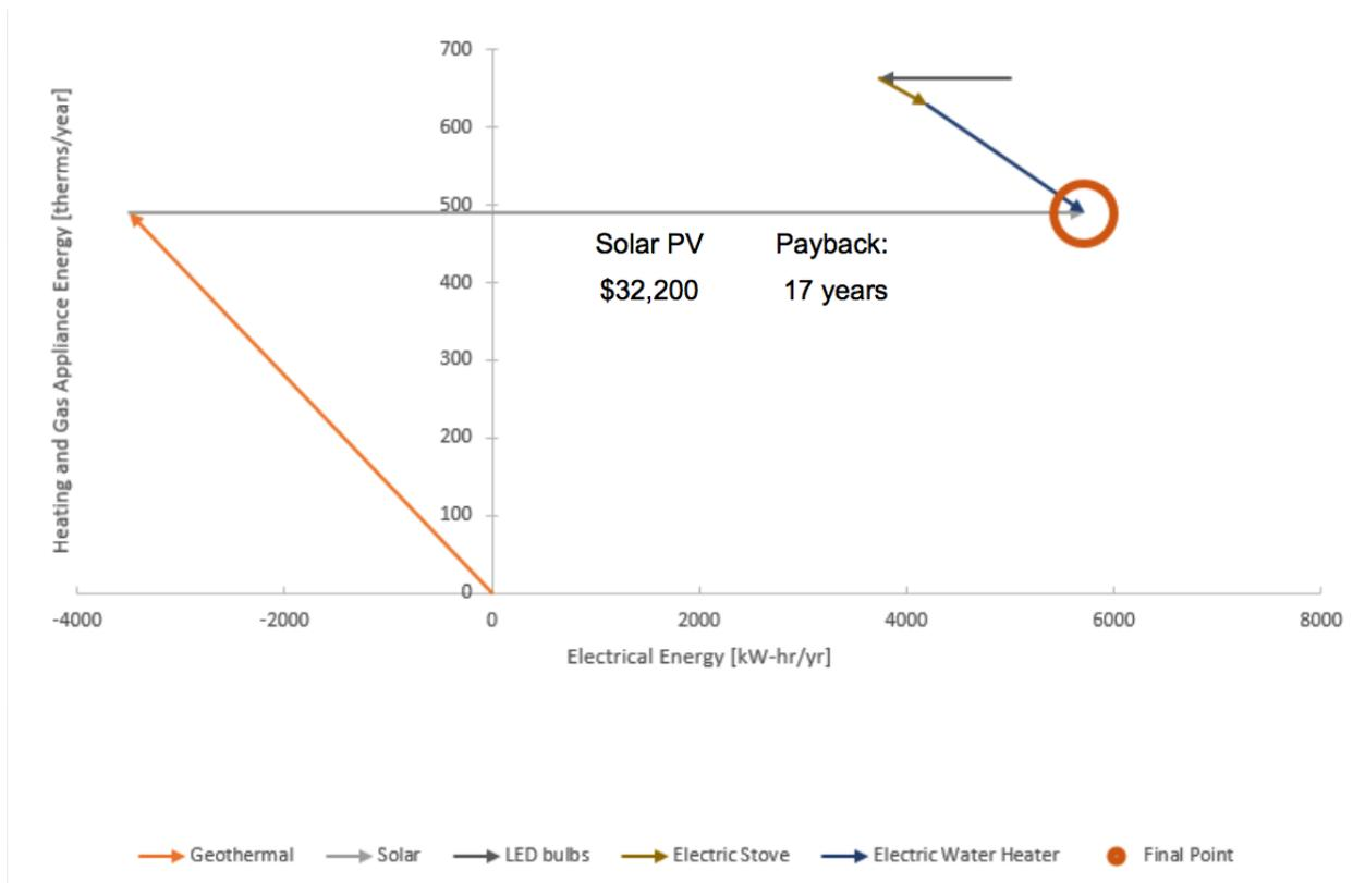
Figure A11: Effects of Solar PV
