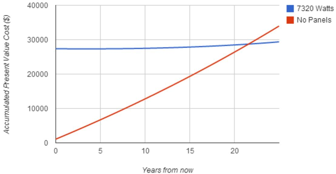
Figure A7.A9 Initial cost and payback period of a considered solar panel
