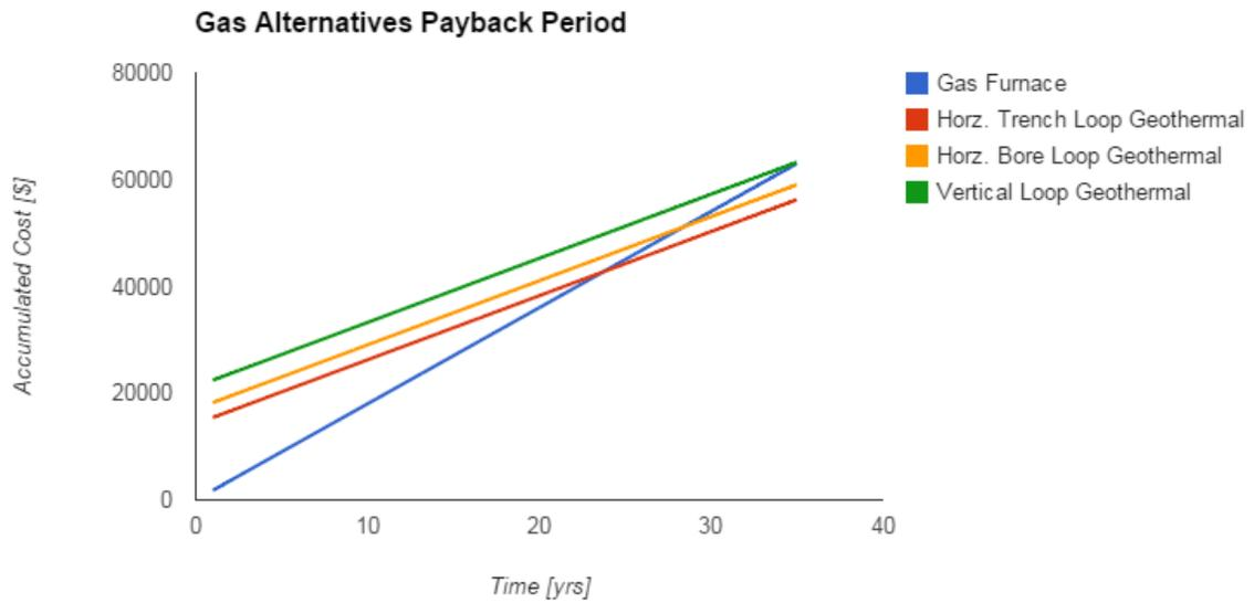
Figure A7.A13 Payback Period for Geothermal Alternatives
