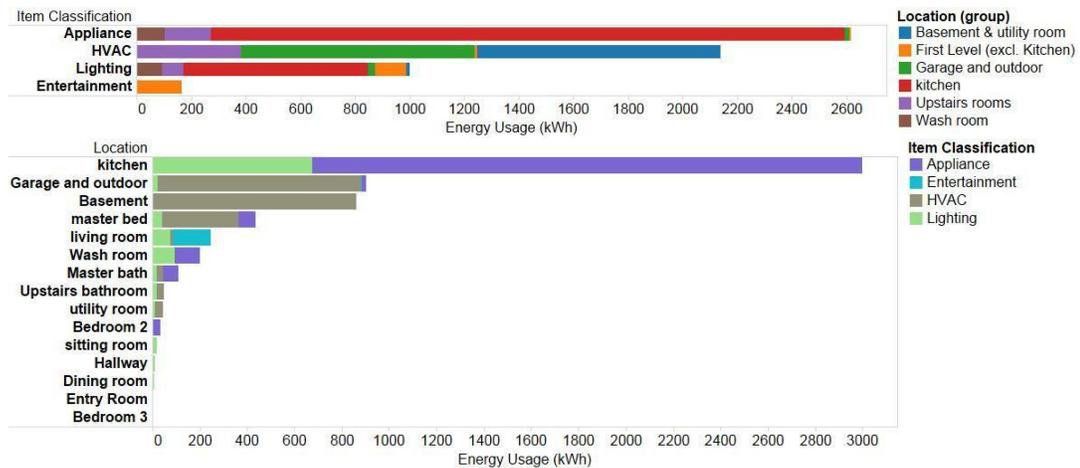
Figure A12: Electric Energy Breakdown
