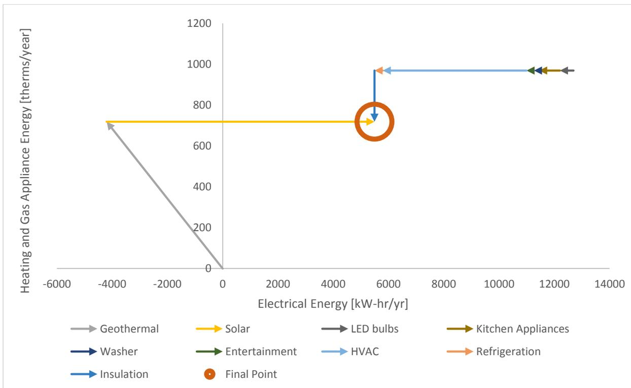
Figure 13. Final overlay plot with reduction implementations
