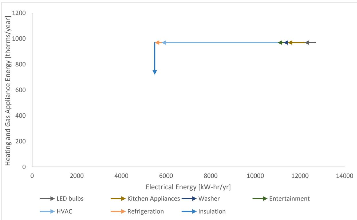
Figure 25. Insulation Implementation
