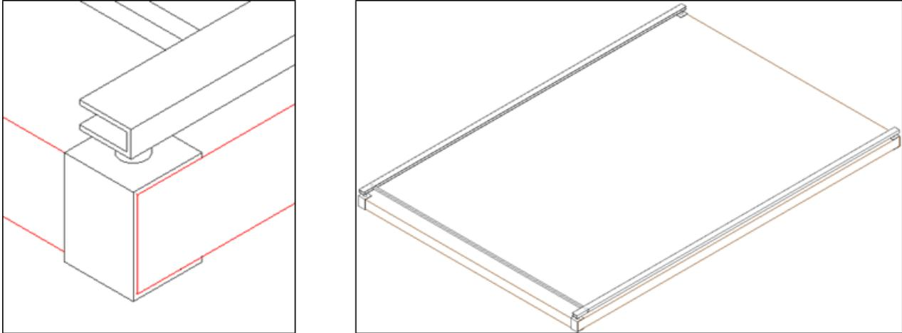
*Figure C6-56. Overall view and close-up of snow removal device.*
