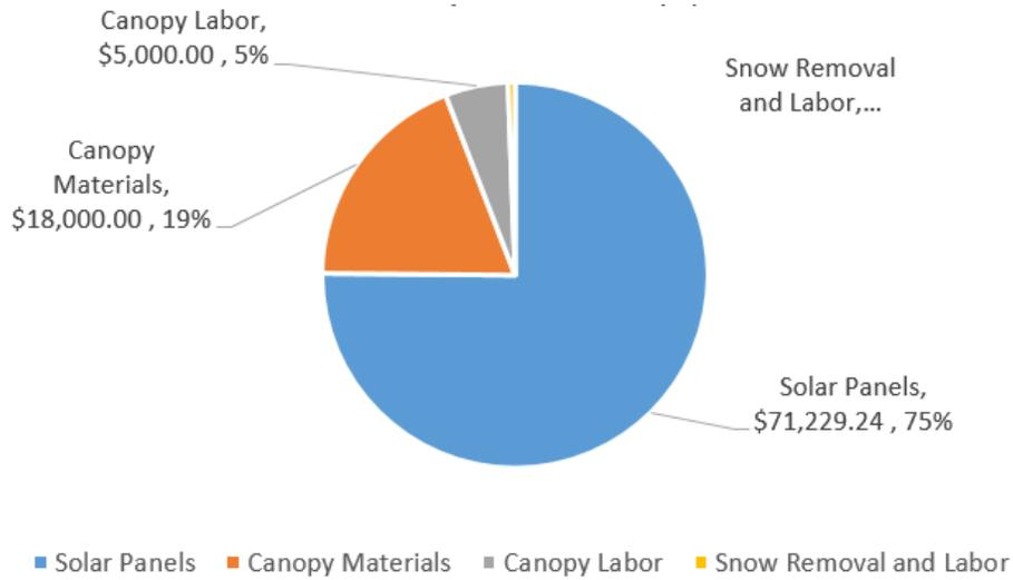
Figure 39 Cost of Solar Panel System
