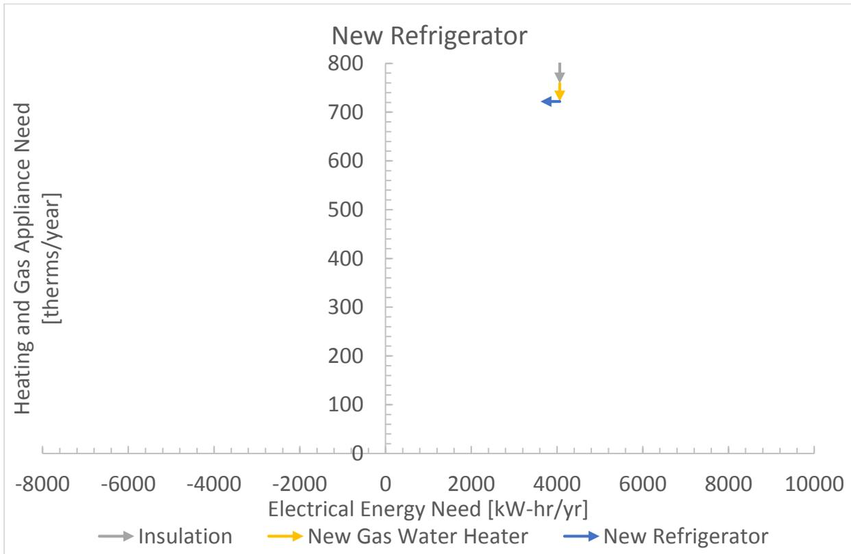
**Figure 8:** Annual energy need reduction after refrigerator replacement
