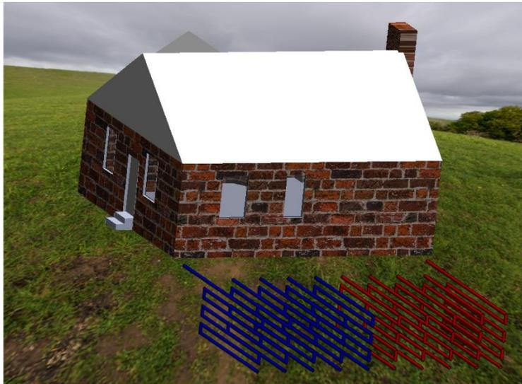
**Figure 9:** Geothermal field model mock-up. (Note: proposed geothermal field would be vertical, image is shown to illustrate location and general piping layout).
