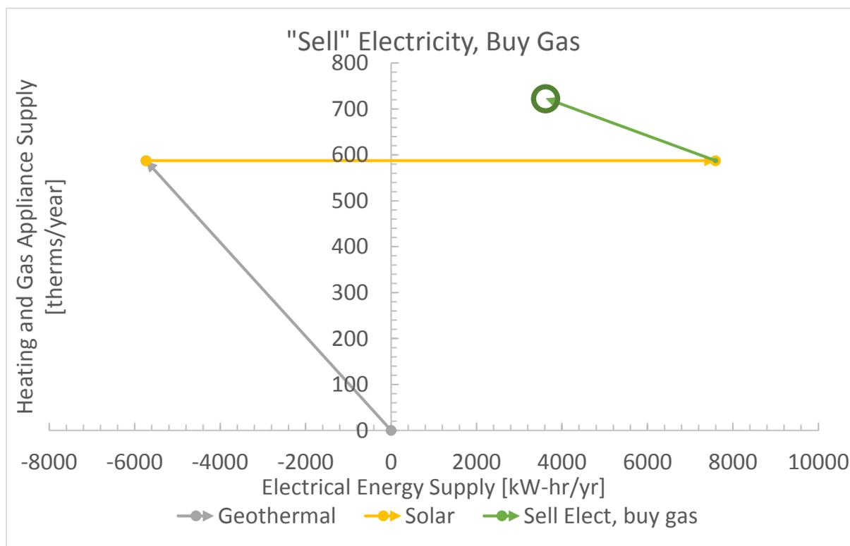
**Figure 13:** Annual energy production after electricity-gas exchange
