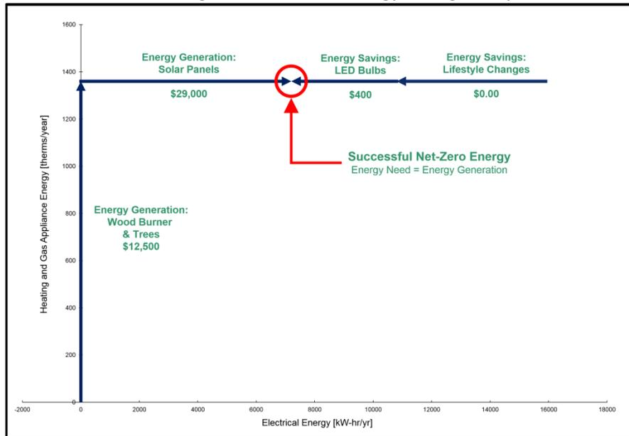
Figure 47 Graphical Net Zero Plan
