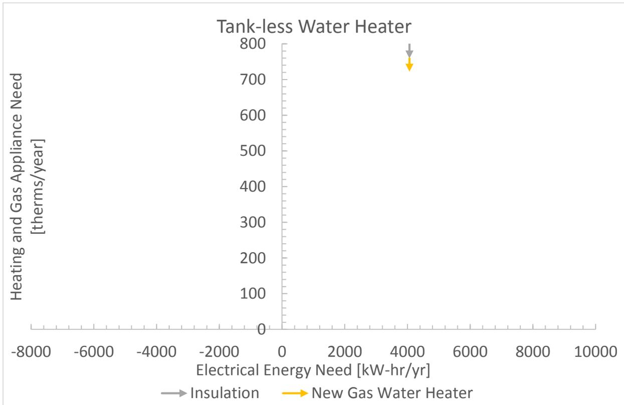
**Figure 7:** Annual energy need reduction after water heater replacement
