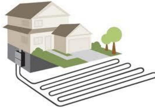
Figure 6 – Horizontal Geothermal Heat Pump
