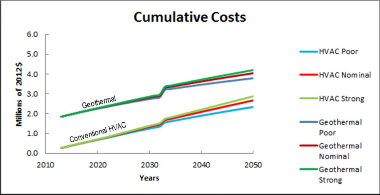
Figure F-4: Cumulative costs for both the conventional HVAC and geothermal systems
