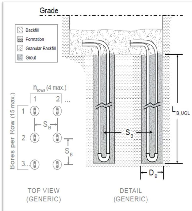
Figure D-4: Cross-Sectional View of Bore
