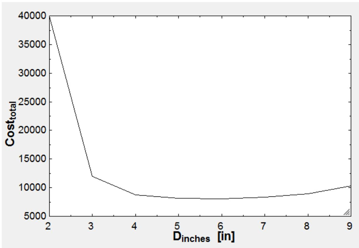
Figure C-5: Total transport cost for a bore field located 690 meters away from the West Wing. The total cost is dependant on the diameter of the pipe; minimum cost is for 7 inch pipe.
