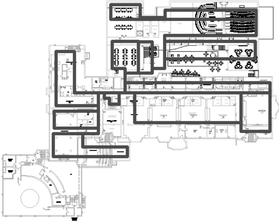
Figure E-1: First floor plan and ductwork design
