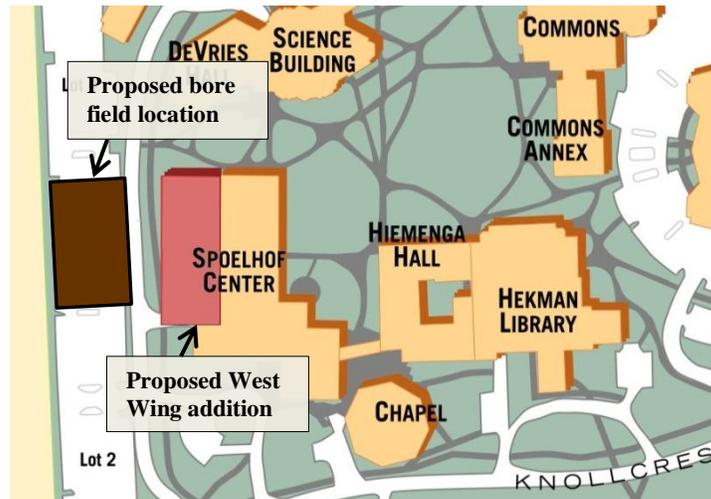
Figure C-2: Locating the bore field in Lot 3 minimizes transport costs and reduces construction impact.
