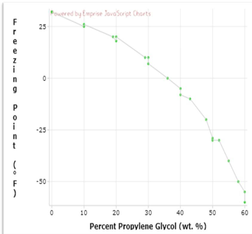
Figure D-3: Geothermal Loop Fluid Freezing Point as Weight Percent of Propylene Glycol Increases
