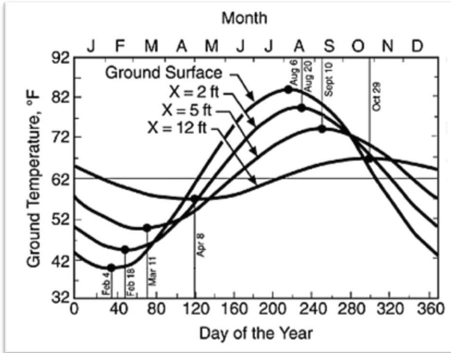
Figure D-2: Sinusoidal Temperature Gradient at Various Depths
